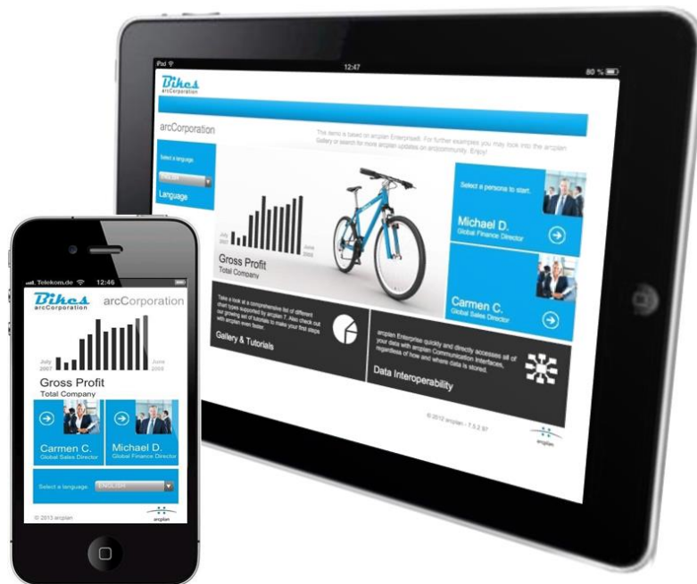
Figure 8: Example for responsive web design: the mobile version of arcplan 8. A dashboard automatically fits to the different screen dimensions of a smartphone and a tablet, and it also supports the different navigation controls.
